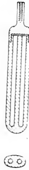
FIG. 233.—Silver screen 1 mm. thick adapted to contain two tubes side by side and fitted with screw terminal.
